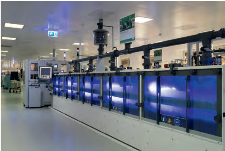
Etching technology process of ISA-PLAN® resistors
