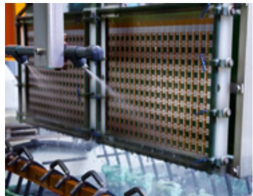
Plating process in new panel plating shop
