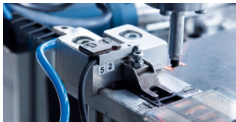
Components are comprehensively tested, measured and calibrated before packing in standard tapes and reels
