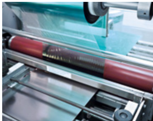
Laminating resistor substrates in cleanroom
