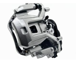
With an EPB, the switch in the car's interior starts up the actuator, which presses the brake pads against the brake discs. The control unit is set up with a fixed current profile for the EPB's contact pressure, which monitors the shunt when the EPB is activated. Image: ©Shutterstock
