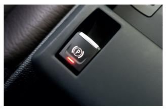
The touch of a button is all that's required to activate the electronic parking brake and safely park a vehicle at any location, even on an incline. Image: ©Shutterstock
